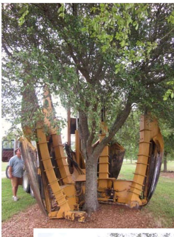
*Ducote's ninety-inch tree spade that can move a 13,000 pound chunk of dirt from around the tree—5 1/2 feet deep and 8 feet across.*
